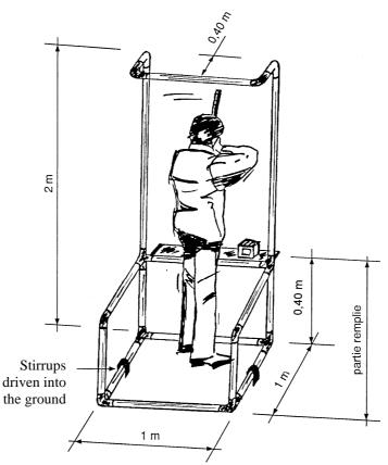
Shooting stand made of coloured P.V.C. tubes, ⊙ 50 mm Straight tubes + interlocking elbows. All the lower elements are filled with water or sand, or fixed to the ground.
